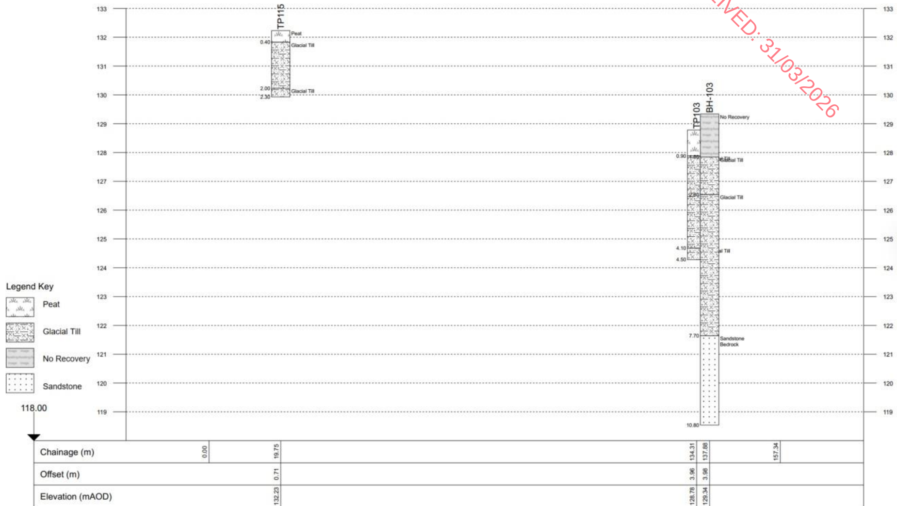
Figure 3-6: WTG4 geotechnical cross-section
